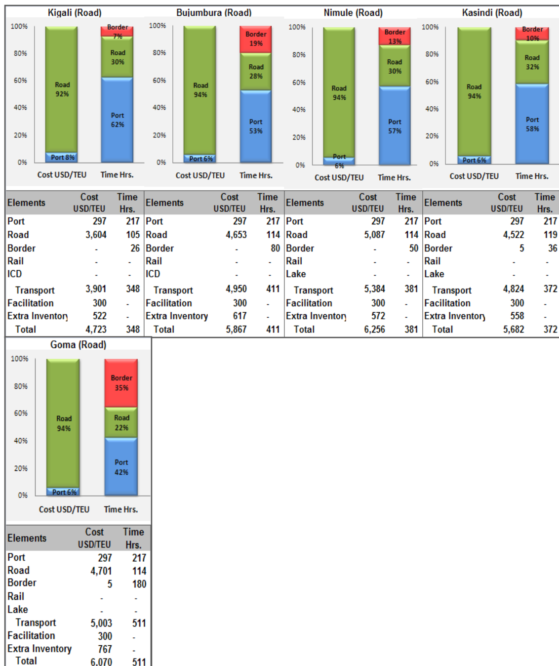
Figure 2-9. Cost and Time for Northern Corridor Destinations Served Only by Road Transport - Imports, 2010 (light containers)
