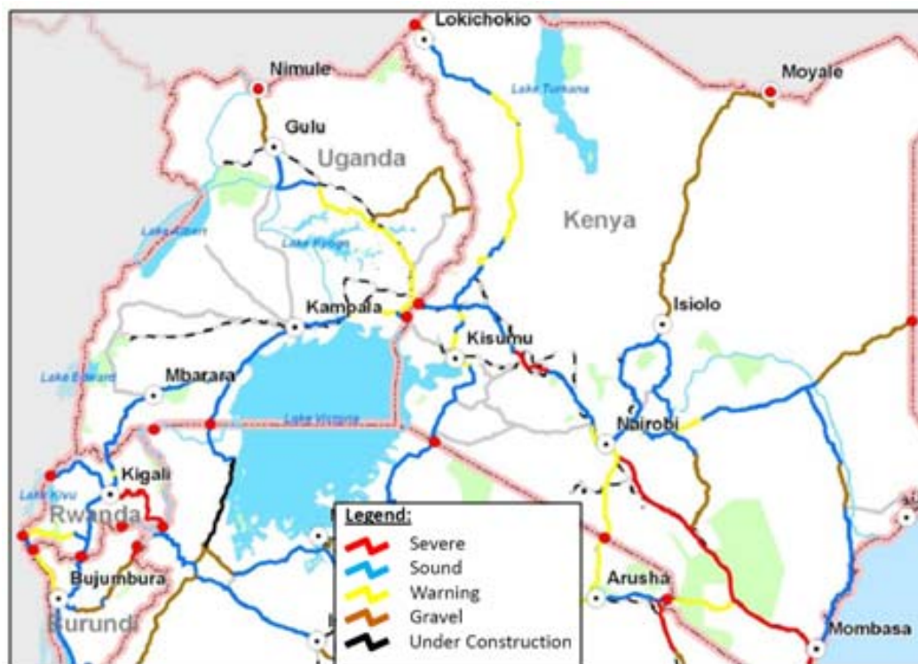
Figure 2-5. Condition Assessment of Northern Corridors Roads
