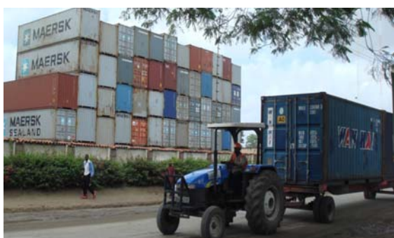
Figure 5-1. Use of Tractor for Container Transfers
