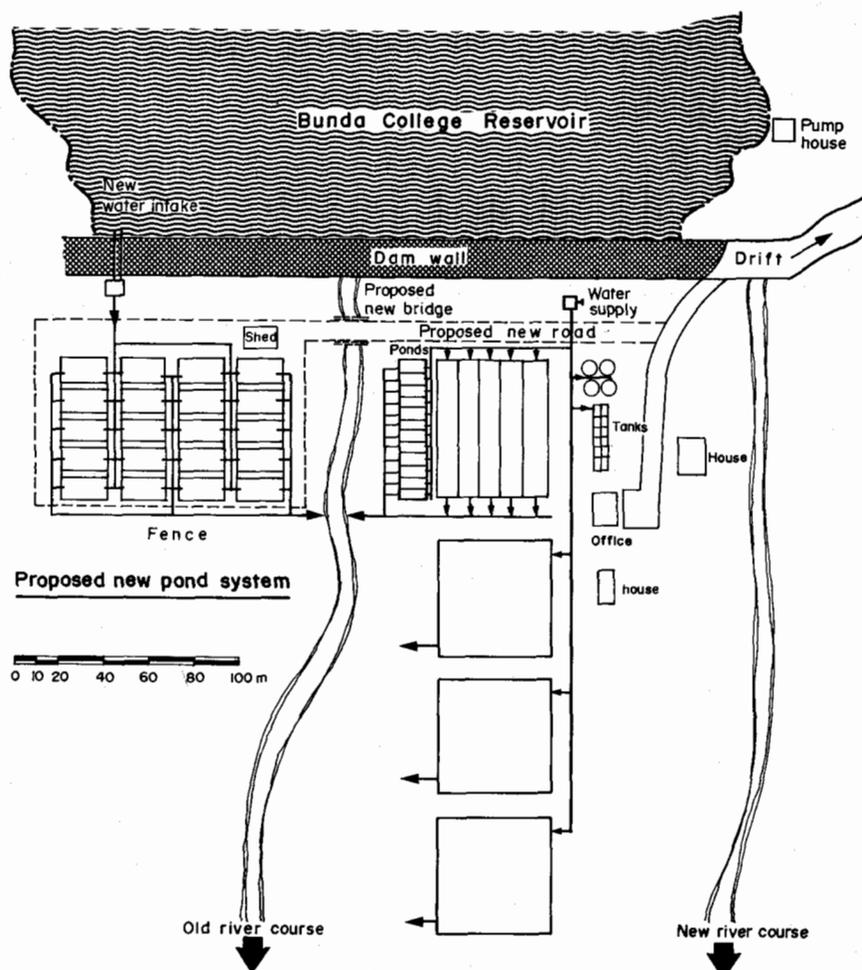
Fig. 7.10. Suggested layout of the ICLARM/GTZ-FD-UM Collaborative Fish Farming Project and 20 x 200 m<sup>2</sup> research ponds at Bunda College of Agriculture, Malaŵi.
